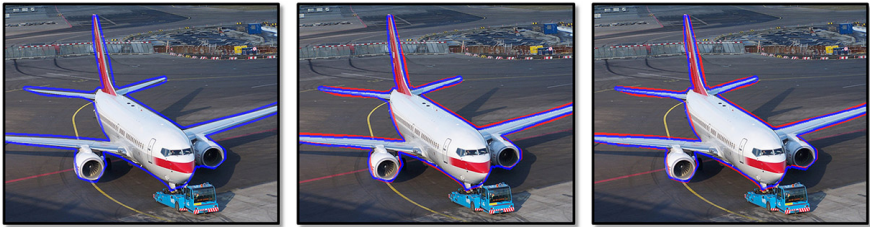
Fig. 2. Evolution of edge alignment during training (progression from left to right). Blue color indicates the aligned edge labels learned by SEAL, while red color indicates the original human annotation. Overlapping pixels between the aligned edge labels and the original annotation are color-coded to be blue. Note how the aligned edge labels gradually tightens around the airplane as training progresses. Best viewed in color.
